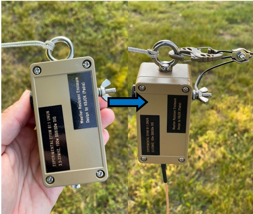
Figure 19: Establish your girth hitch first, then attach the 20m wire element to the UNUN.
