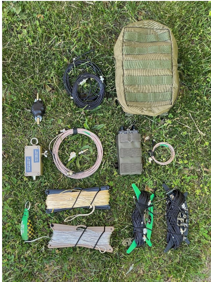
Figure 18: K8JOK's antenna kit. From top left to lower right, Packenna RF choke, Ed Fong dual band J-pole, 10"x6" MOLLE pouch, 81:1 UNUN, 25' RG-316 coax, miscellaneous adapters for the J-pole, MAT-10 antenna tuner in a MOLLE pouch, 3' RG-316 jumper, 14oz throw weight, 180' & 90' arborist throw line on winders, linked EFHW wire elements on winders, 20/30/40m elements on one winder and 60/75/80m elements on the other.
