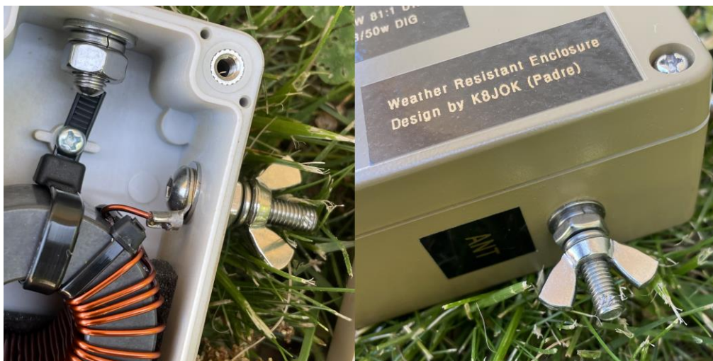
Figure 12: Detail view of the antenna stud. Note the orientation and 90-degree bend in the ring terminal attaching the core to the stud.
