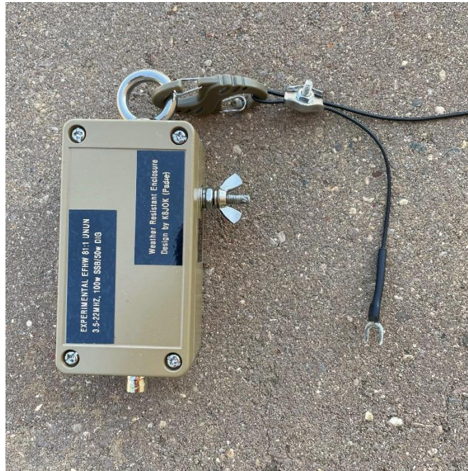
Figure 16: Completed fork spade terminal connection for 20m element.
