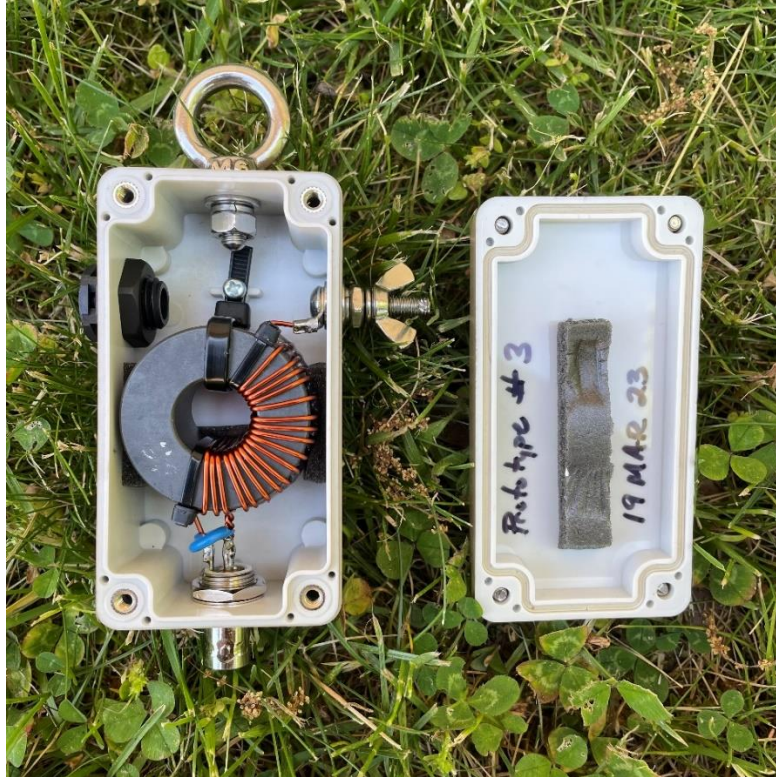
Figure 11: The completed UNUN ready for final assembly. Carefully note the placement of each component before cutting and soldering.
